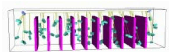
Figure 6: A wireframe bounding box encloses the workspace. ClosestVE uses a straightline local planner to connect small robot block configurations perpendicularly to the single pre-existing roadmap edge passing from left to right over the large vertical obstacle walls.
