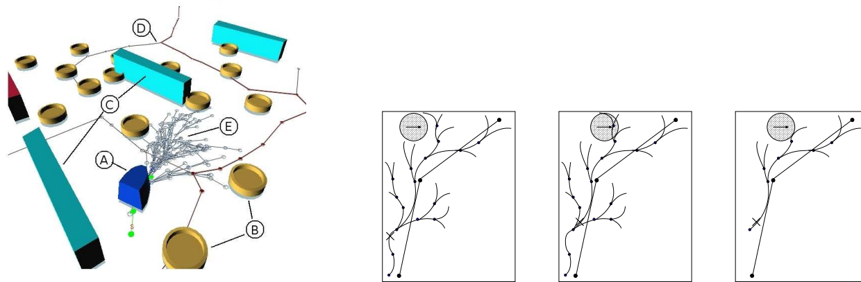
Figure 1: A test environment showing different aspects considered in our planning framework. These aspects include (a) a robot, (b) soft objects (other agents), (c) hard objects (moving and static), (d) a global-dynamic roadmap and (e) kinodynamic local plans (also showing the update step on the right).
